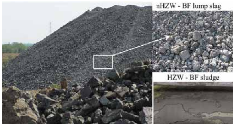
Fig. 2. Layout of hazardous waste (sludge) and non-hazardous waste (slag) which will be disposed at the landfill
