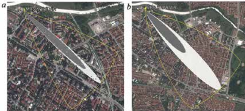
Fig. 4. Consequence maps: flammable area of vapour cloud (a), and vapour cloud total area (b)
