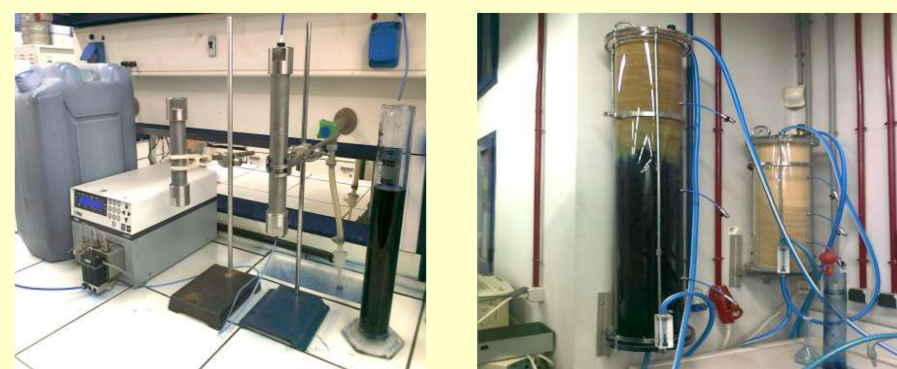
Figure 4: Adsorption columns (top) of stainless steel at lab/bench scale and (bottom) of polymethylmethacrylate (PMMA) at Pre-pilot (in the right hand side) and pilot scale, adsorbing methylene blue on modified biomass.
