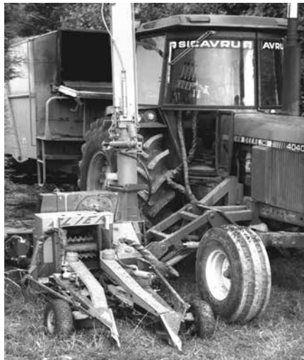
Fig. 3. CLIER harvester mounted on a tractor
