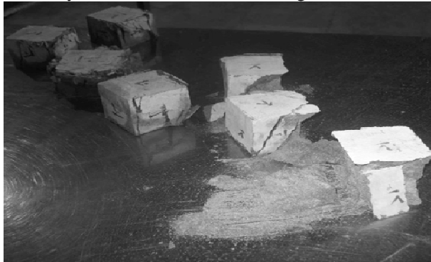
Picture 2-broken samples without fiber addition.
